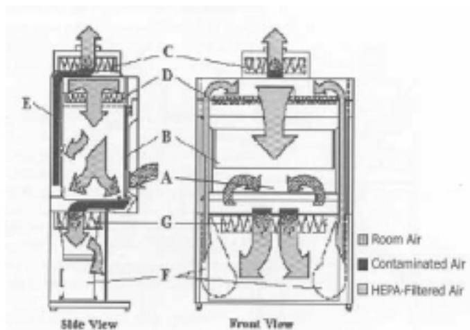
Connection to building exhaust system required.
