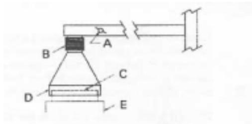
**Thimble unit for ducting a Class II, Type A BSC.**
